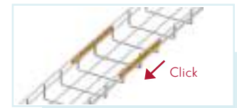
Cable trays locking with ergots
